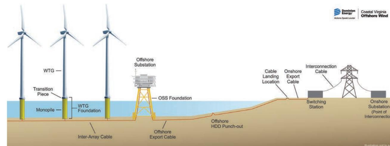
Offshore wind farms require substations and hundreds of miles of submarine transmission cable. Source: Dominion Energy
